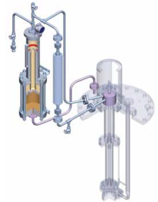
Vertical pump arrangement
